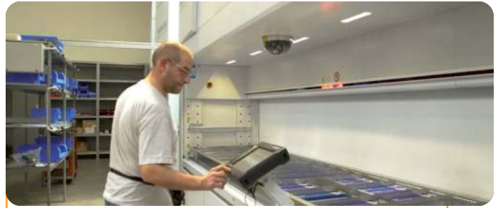
Put-to-light systems connected to WMS
